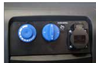
Synchronized start-up when connecting a machine to the vacuum cleaner
