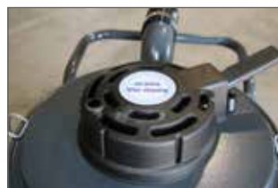
Pulse jet filter cleaning system
