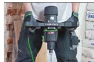
Wide and ergonomic frame, raised centre of gravity
