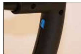
Electric speed controller to adapt speed
