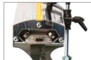
Guide rail equipped with an interchangeable stainless steel track
