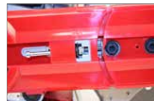
Easily accessible belt tensioner
