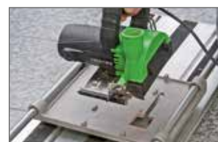
Quick and tool-free attachment of the saw to the cutting table
