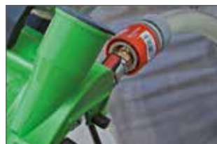
Direct connection to the water inlet with flow rate adjustment
