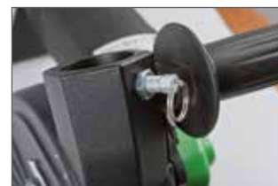
Locking of the suction hose, prevents accidental release during grooving
