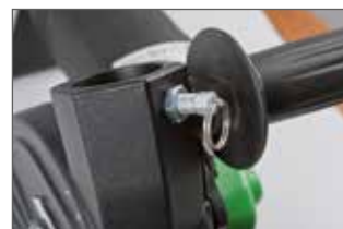
Blocking of the suction hose, prevents accidental release during grooving
