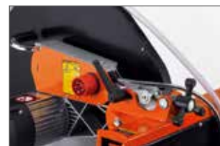
Adjustment of cutting depth by handwheel
