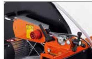
Cutting height adjustment with a knob and a locking lever
