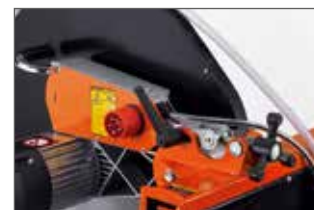
Cutting depth adjustment by handwheel
