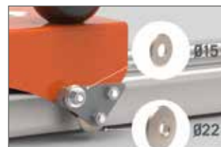
2 wheels: \varnothing 22 mm (very hard tiles) and \varnothing 15 mm (less hard tiles)
