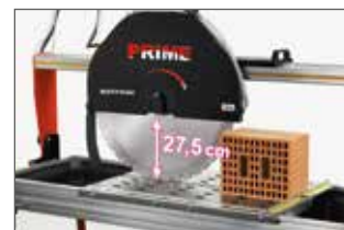
Cutting depth 275 mm
