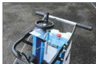
Cutting depth adjustment by handwheel
