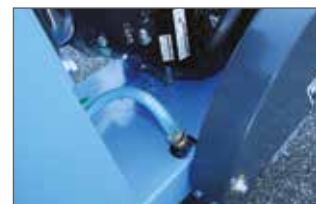
Hose placed at the back of the casing = no damage
