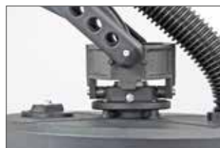
Articulated anti-vibration system mounted on springs = compensates for irregularities
