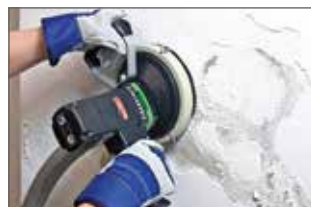
Direct connection to vacuum cleaner for improved dust extraction
