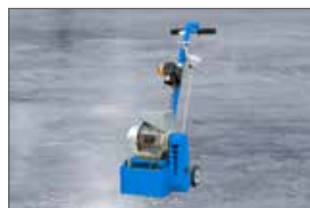
Use: floor marking, removal of residues (marking, glue, paint)
